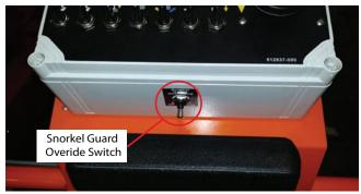
Figure 3-5: Snorkel Guard Overide switch
