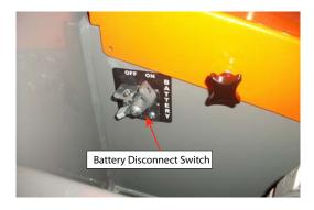
Figure 2-2: Battery Disconnect Switch
