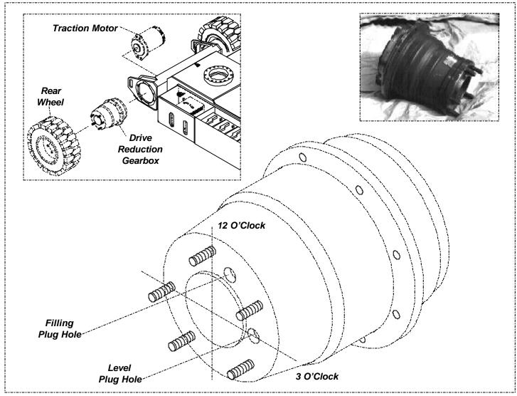
Figure 4-14: Drive Reduction Gearbox
