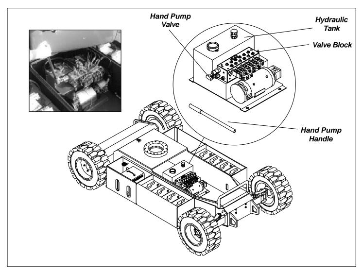
**Figure 3-4: Manual Telescopic Retraction**
