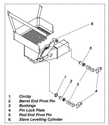
Figure 4-21: Slave Levelling Cylinder
