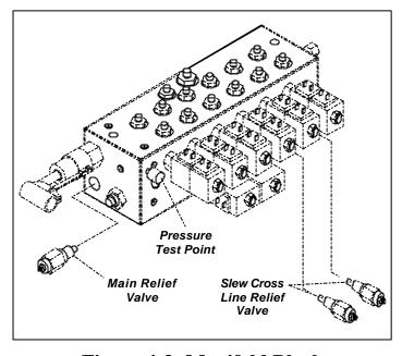
Figure 4-3: Manifold Block
