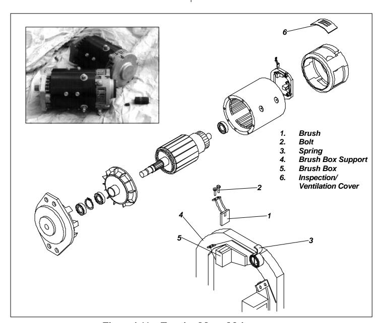
**Figure 4-11: Traction Motor Maintenance**
