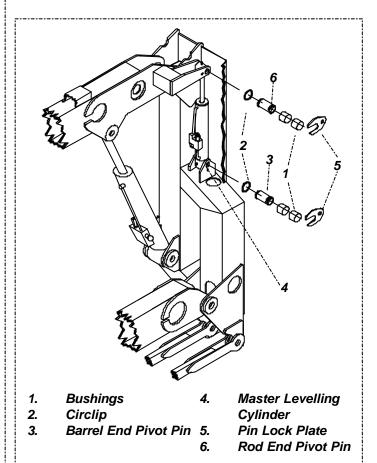
Figure 4-20: Master Levelling Cylinder
