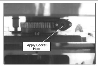
To rotate the Elevating Assembly first apply a 7/8" socket wrench to the shaft and turn to rotate the Elevating Assembly. When finished remove the wrench.
