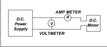
Figure 4-12: Electrical Test Circuit
