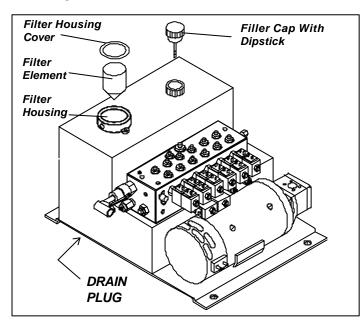
Figure 4-2: Oil and Filter Replacement
