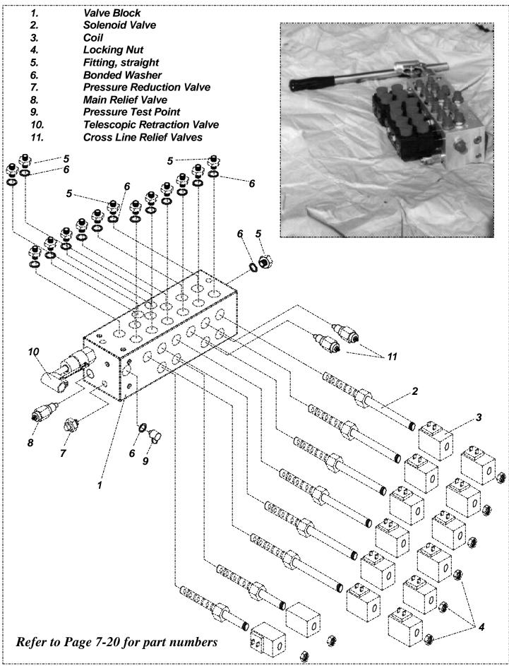
Figure 4-9: Manifold Block Components
