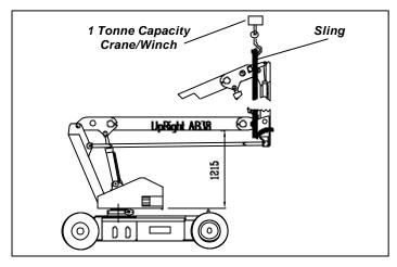
Figure 4-6: Supporting Elevating Assy.
