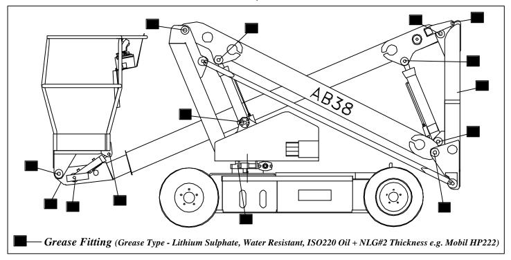
**Figure 4-1: Lubrication Points**
