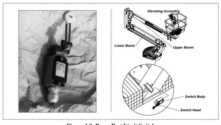
Figure 4-8: Boom Rest Limit Switch
