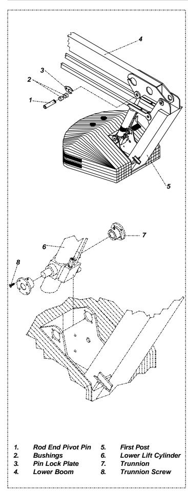
Figure 4-15: Lower Lift Cylinder
