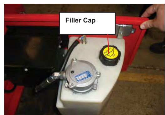
Figure 8: Hydraulic Fluid Reservoir and Dipstick
