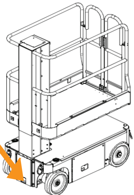
FIGURE 2-7: Emergency lowering valve
