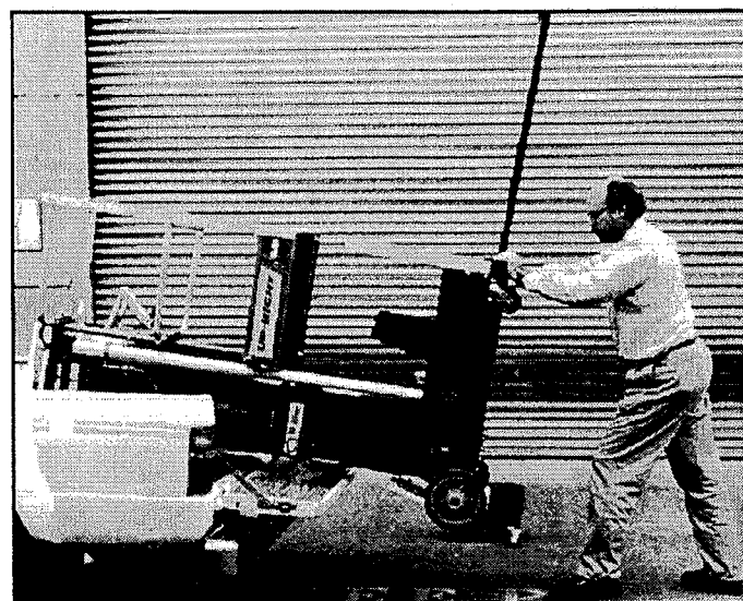
Figure 3-12: Pushing machine into transport position
