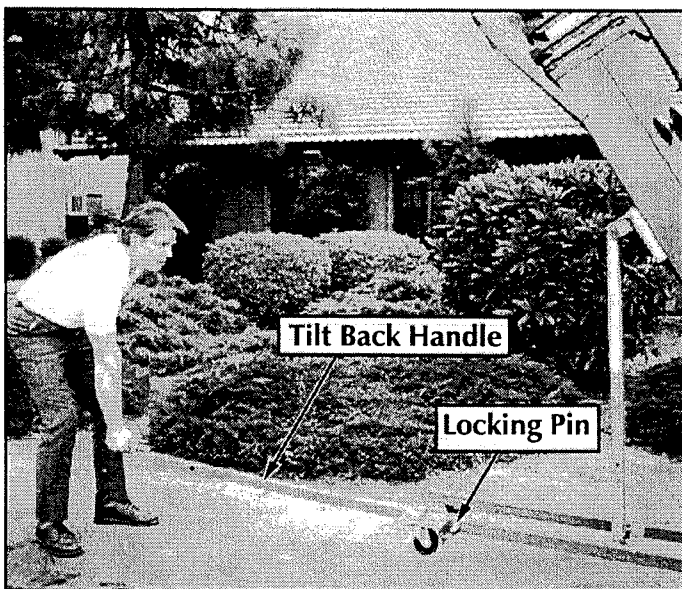
Figure 3-14: Lowering and raising machine with Tilt Back Handle
