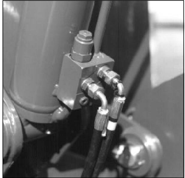
The Overcentre Valves are located towards the Rod End of the Lower Lift and Upper Lift Cylinders.
