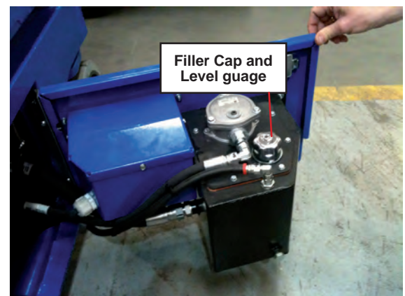
Figure 8: Hydraulic Fluid Reservoir and Dipstick
